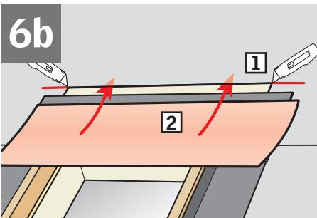
**ENGLISH:** To allow for proper drainage, interweave roofing underlayment as shown in **6a** for new construction applications. For retrofit applications, interweave roofing underlayment as shown in **6b**.
