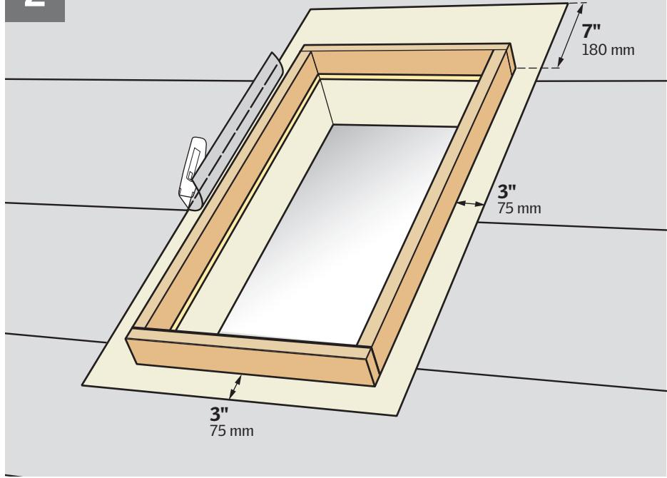
**ENGLISH:** To ensure waterproofing, skylight curbs shall be completely wrapped in VELUX adhesive skylight underlayment as indicated. Underlayment must be applied before installing the flashing. Remove existing roofing underlayment around the rough opening as shown.
