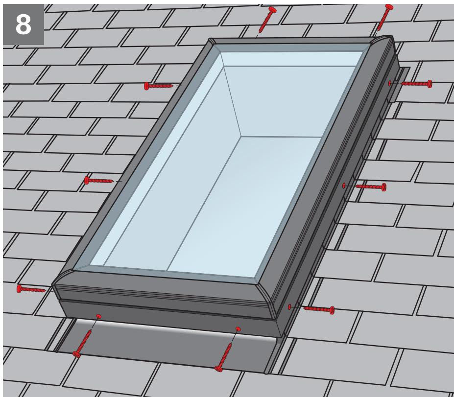
**ENGLISH:** Center the skylight on top of the curb and secure with #8 1 $\frac{1}{4}$ " (45 mm) pan head stainless steel screws provided. Screws will penetrate the curb by at least  $\frac{3}{4}$ " (19 mm).
