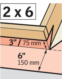
**ENGLISH:** Wrap the bottom and the corners of the skylight curb with the underlayment and create water-shedding laps over roofing underlayment.
